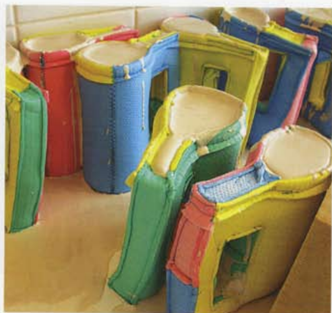
Top: A series of approximately 50 mould experiments. Above: Casting in some of the moulds.
